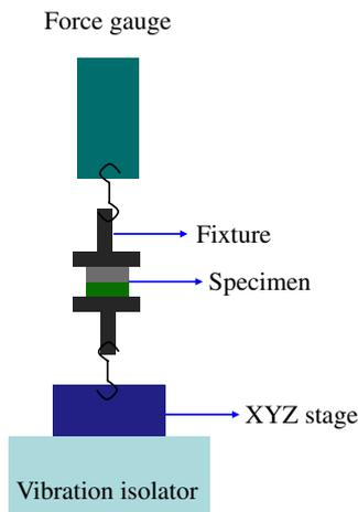
**Figure 9.** A pull-test setup to measure the interlocking force of connectors and sockets.
