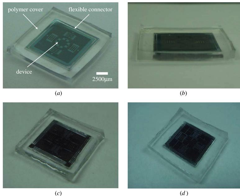
**Figure 8.** The polymer cover with different connector designs and the MEMS device chip after packaging.
