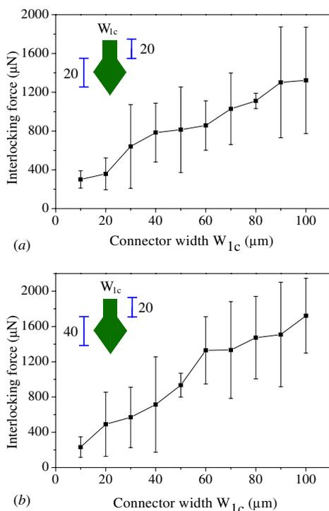
**Figure 10.** Measurement results of interlocking force for a pair of connectors and sockets at a different connector width  $W_{1c}$ . The connector and socket are of the same dimension, and (a)  $L_{1c} = L_{1s} = 20 \mu\text{m}$  and  $L_{2c} = L_{2s} = 20 \mu\text{m}$ , and (b)  $L_{1c} = L_{1s} = 20 \mu\text{m}$  and  $L_{2c} = L_{2s} = 40 \mu\text{m}$ .
