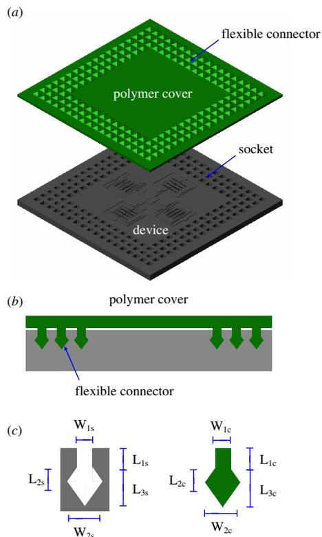
**Figure 1.** Schematic illustration of the present concept: (a) polymer cover and MEMS device before packaging, (b) packaging of the polymer cover and the MEMS chip using the interlocking of flexible connectors and silicon sockets and (c) tunable dimensions of the present connectors and sockets.
