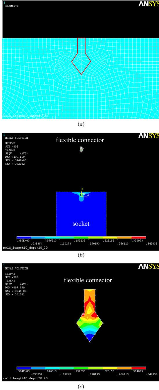
**Figure 3.** Mechanical characteristics predicted by the finite element simulation: (a) the typical finite element model; the typical stress distribution during demolding for (b) silicon socket and (c) flexible connector.
