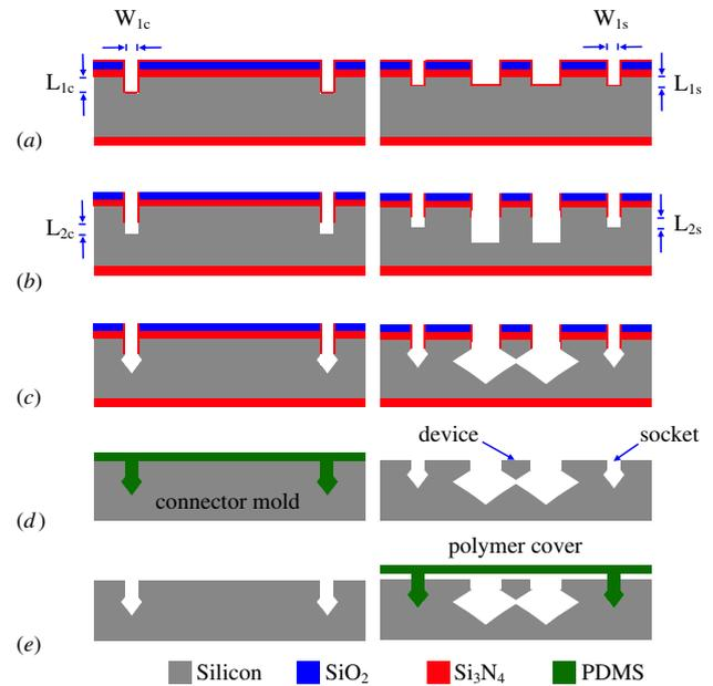
**Figure 5.** The present fabrication process steps.
