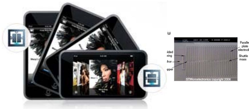
Movements control the action using MEMS accelerometer
