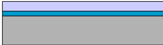
Cast a thick resist layer (PMMA)
