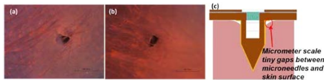
Fig. 9. Fluorescent images of mouse skin: (a) Texas red and nano-fluorescent beads are delivered with microneedle device without CNT nanofilters; (b) Texas red and nano-fluorescent beads are delivered with microneedle device with CNT nanofilters; (c) The micrometer scale gaps occur between skin and bottom edge of a microneedle due to skin deformation.
