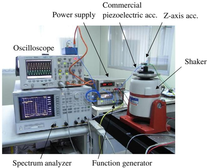
Figure 7. The measurement setup to characterize the performance of the accelerometer.
