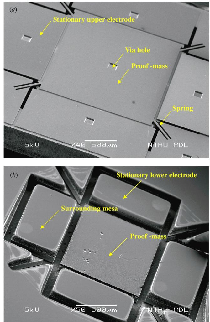
**Figure 4.** The SEM micrographs of a typical fabricated accelerometer where (a) the front-side view shows the components made of the device Si layer, and (b) the backside view shows the components made of the handle Si layer.
