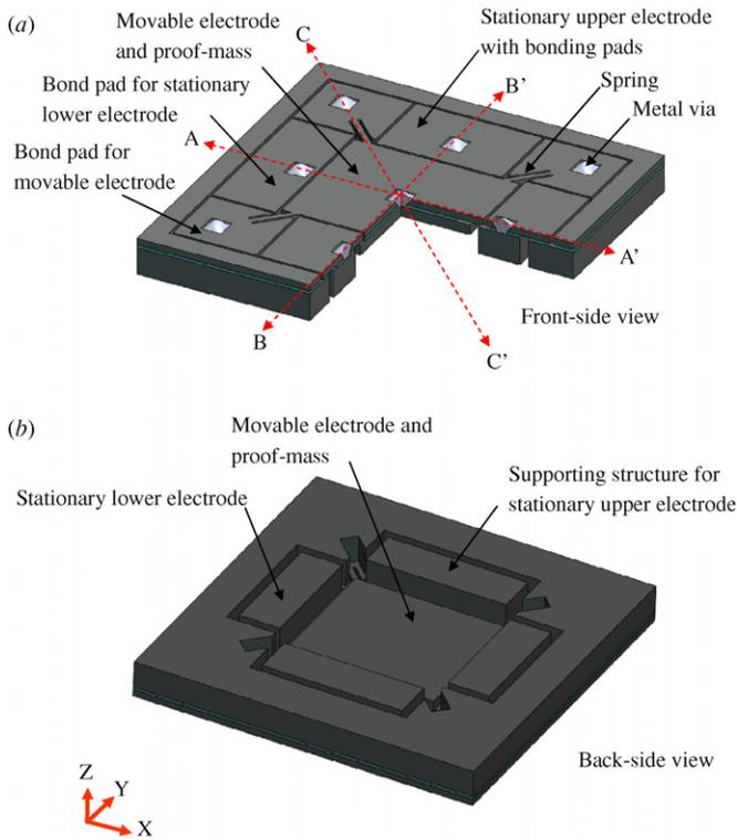
**Figure 1.** The schematic illustrations of the present Z-axis SOI accelerometer showing (a) the front-side view of the accelerometer formed by the device Si layer of the SOI wafer, the springs, proof mass and movable electrodes, bonding pads and stationary electrodes, and metal-vias, are clearly observed; and (b) the backside view of the accelerometer formed by the handle Si layer of an SOI wafer.
