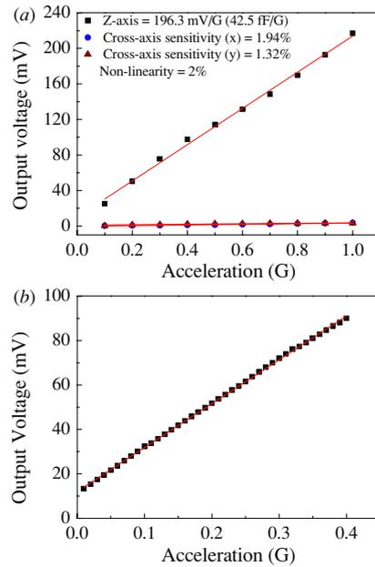
Figure 9. The typical measurement results of (a) the output voltage of the Z-axis accelerometer at different excitations and the cross-axis sensitivities at the measurement range of 0.1–1 G; and (b) the Z-axis accelerometer at the measurement range of 0.01–0.4 G with an increment of 0.01 G each time.
