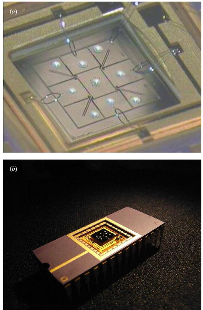
**Figure 6.** The photos show (a) the chip after silver paste dispensing and wire bonding, and (b) the final packaged accelerometer in the ceramic housing.
