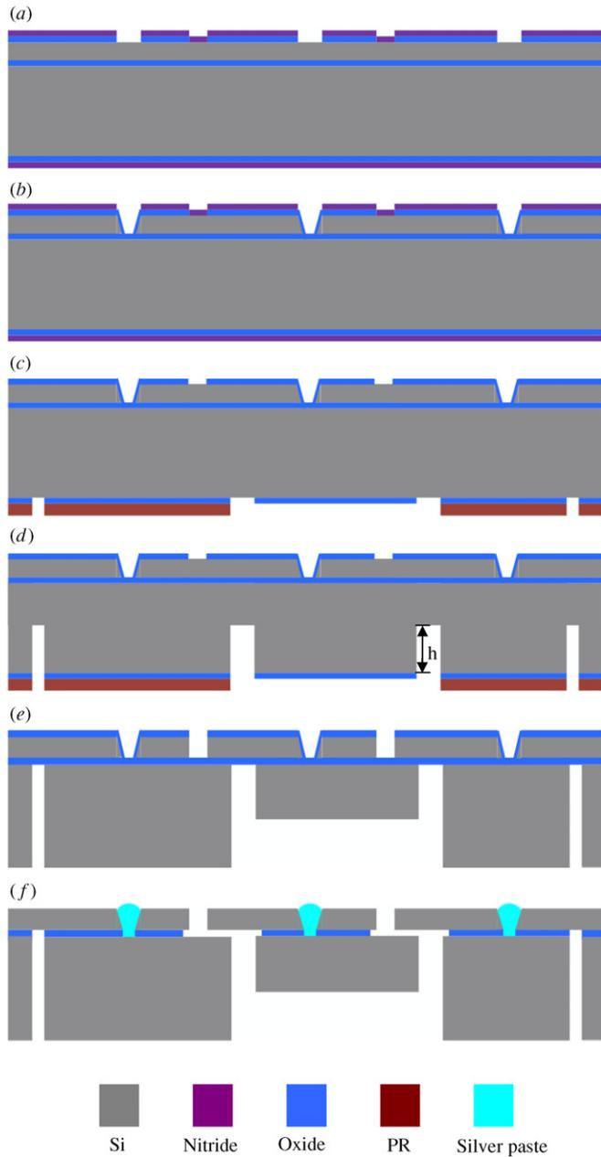
**Figure 3.** The fabrication process steps.
