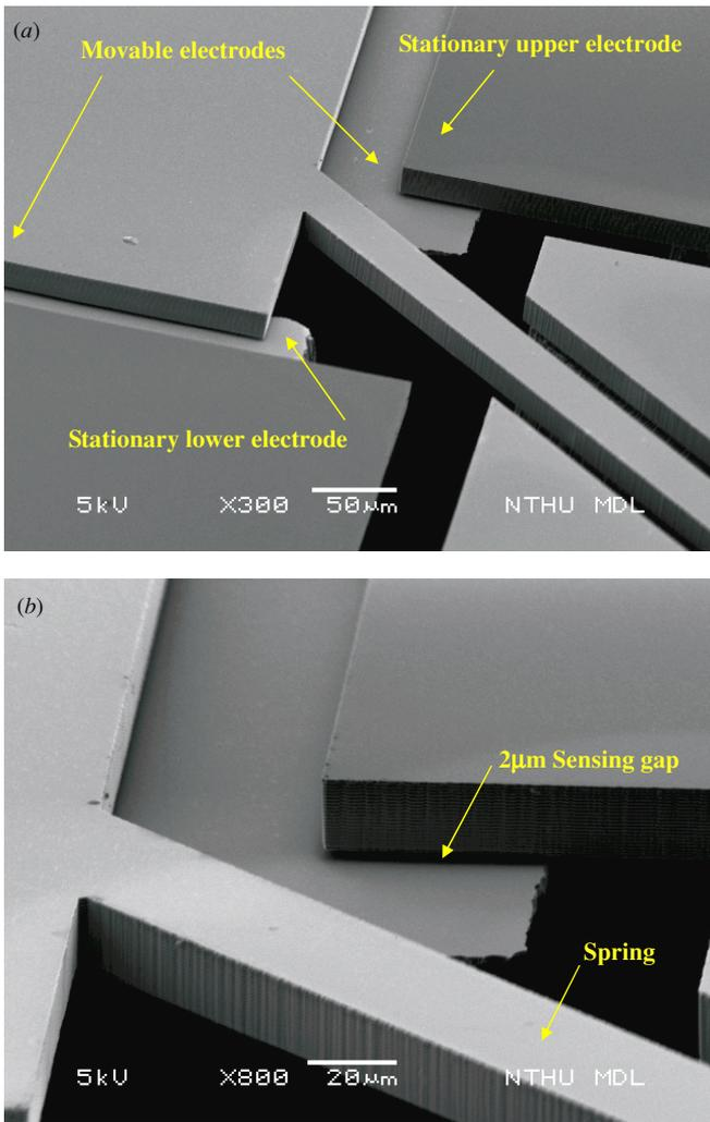
**Figure 5.** The zoom-in SEM micrographs show (a) the differential sensing electrodes, and (b) the gap between the movable and the stationary electrodes.
