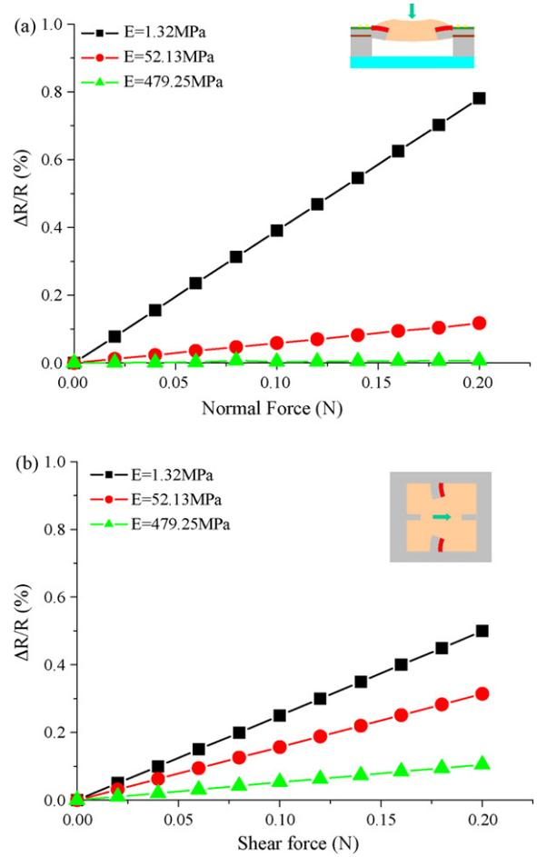
Fig. 4. Typical predicted resistance changes for membranes of different stiffness due to (a) normal load and (b) shear load.
