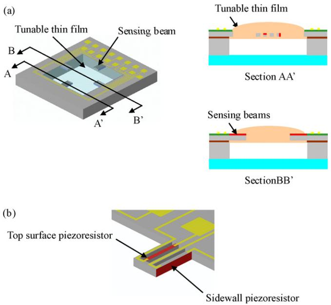
Fig. 1. The schematic illustrations of three axes and thin-film-tunable tactile sensor: (a) the sensor consists of four piezoresistive sensing beams covered with polymer membrane, and the cross-section views of the sensor and (b) zoom in of the sensing beam to show the top and side-wall doping piezoresistors.
