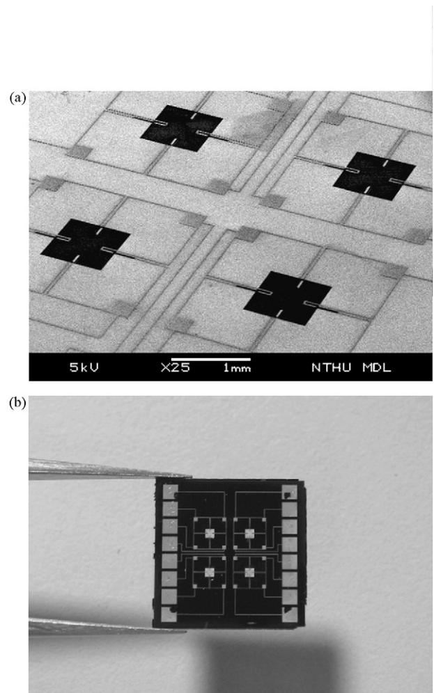
Fig. 12. The SEM photos of a chip with  $2 \times 2$  tactile sensor array: (a) before dispensing of PDMS and (b) after dispensing of PDMS photo.
