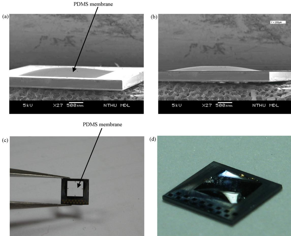
Fig. 8. The photos of typical fabrication results after polymer dispensed: (a) the tactile sensor, (b) the side view photo to show the polymer tactile-bump, (c) the photo to show the transparent polymer membrane, and (d) the completed sensor chip.
