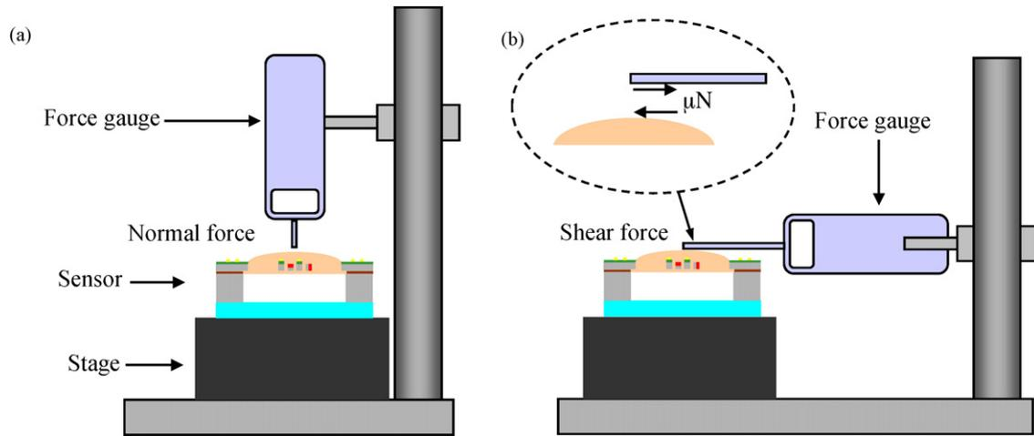
Fig. 10. The experimental setups to measure (a) normal force and (b) shear forces.
