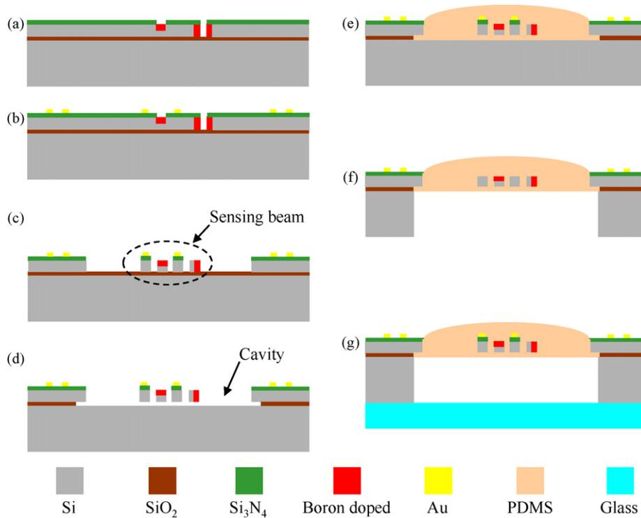
Fig. 6. Fabrication process steps.
