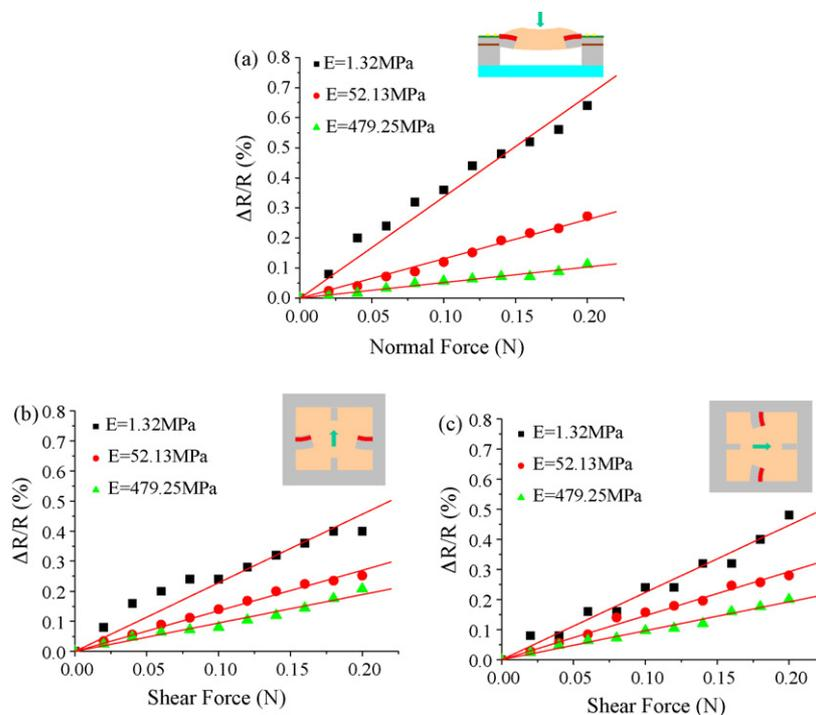
Fig. 11. The measurement results to show the variation of resistance change with (a) normal load and (b and c) shear loads in different directions, and at three different membrane stiffness.
