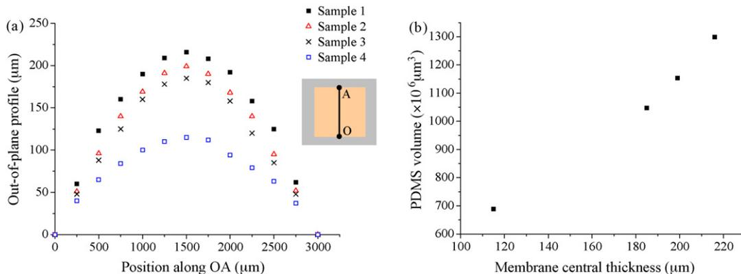
Fig. 9. (a) The typical measured surface profiles of membrane for different volume of the dripped PDMS and (b) variation of the membrane central thickness with the volume of PDMS.
