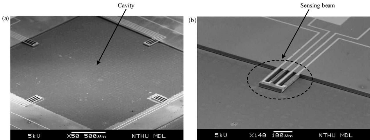
Fig. 7. The SEM photos of typical fabrication results before dispensing of polymer: (a) the sensing unit consists of four sensing beams and (b) zoom-in of a sensing beam.
