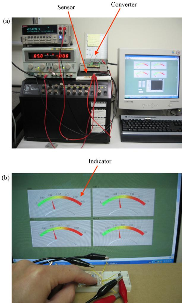
Fig. 13. (a) The test setup to perform the contact test of tactile sensor and (b) the typical measurement result during the test of a  $2 \times 2$  tactile sensor array.
