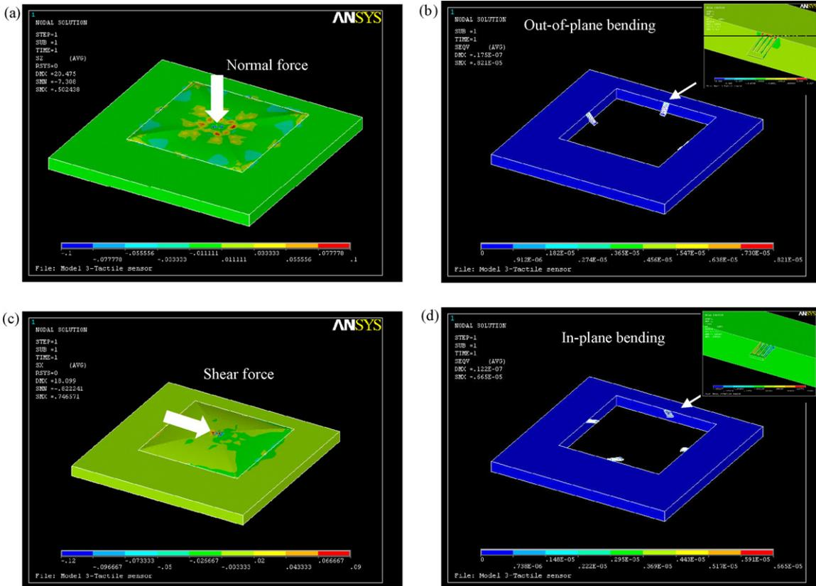
Fig. 3. Typical finite element simulation results to show the stress distribution on membrane and sensing beam after applying (a) normal load and (b) shear load on the present sensor.
