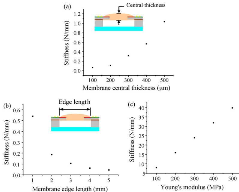
Fig. 5. Typical finite element simulation results to show the variation of membrane stiffness with (a) the central thickness, (b) the edge length, and (c) the Young's modulus of membrane.
