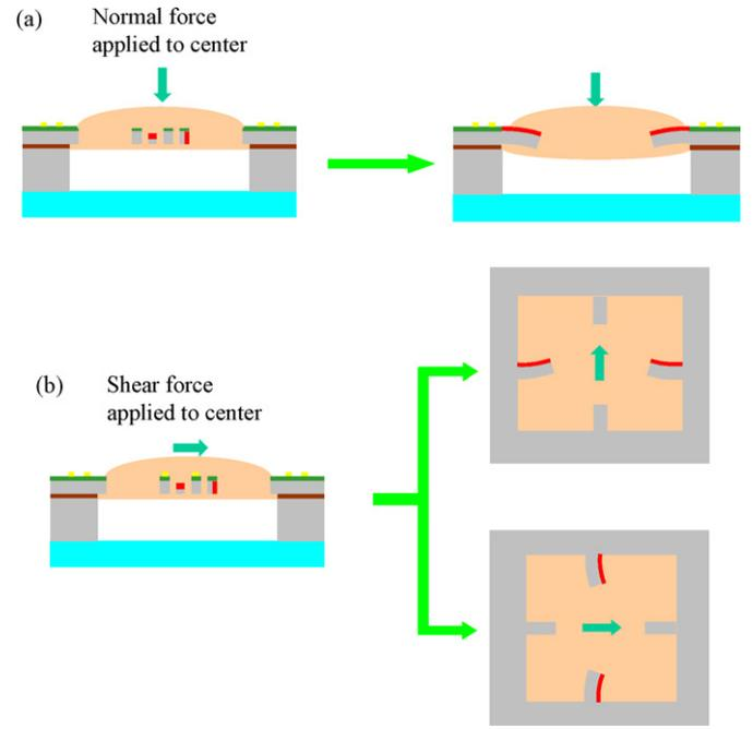
Fig. 2. The schematic illustrations to show the deformation of the polymer membrane and sensing beams resulted from (a) normal load and (b) shear load.
