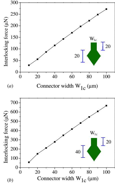
**Figure 4.** Simulation results of interlocking force for a pair of connectors and sockets at a different connector width  $W_{1c}$ . The connector and socket are of the same dimension, and (a)  $L_{1c} = L_{1s} = 20 \mu\text{m}$  and  $L_{2c} = L_{2s} = 20 \mu\text{m}$ , and (b)  $L_{1c} = L_{1s} = 20 \mu\text{m}$  and  $L_{2c} = L_{2s} = 40 \mu\text{m}$ .
