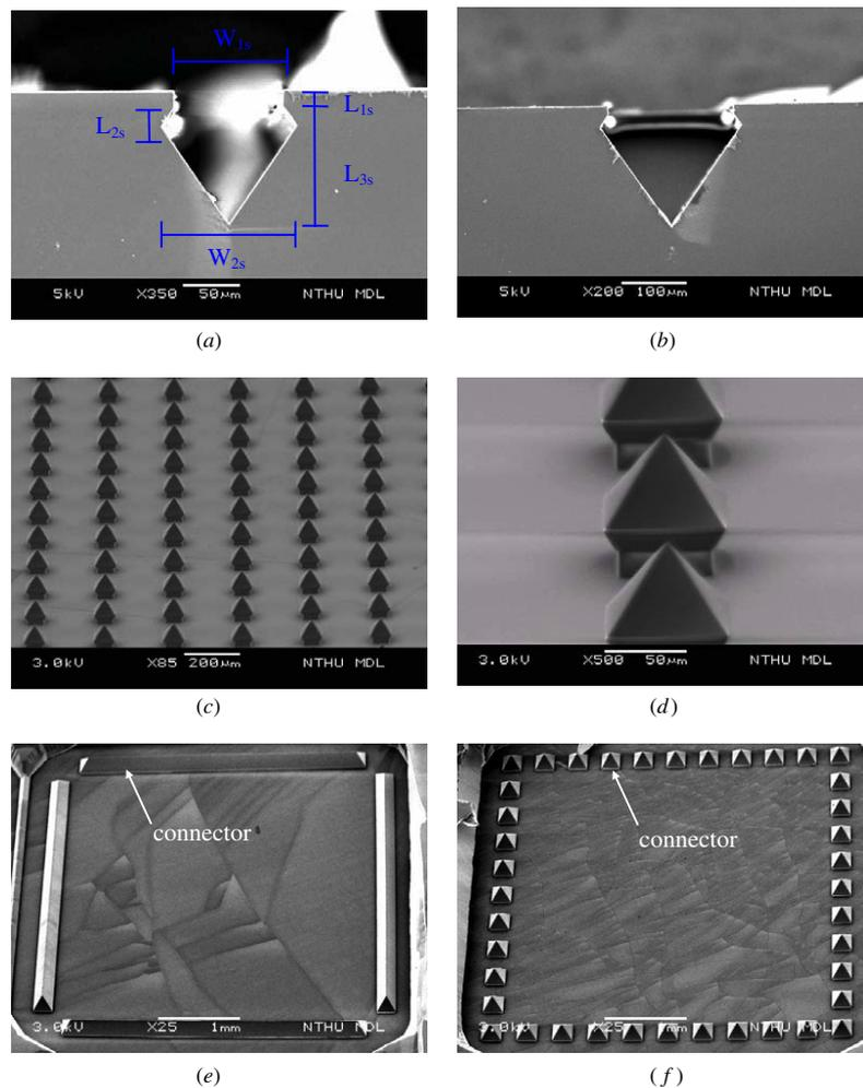
**Figure 6.** SEM micrographs of typical fabrication results: (a) and (b) two different octahedral sockets on the device substrate, (c) the PDMS flexible connector array, (d) zoom-in photo of polymer connector with octahedral tip, and (e) and (f) polymer covers with different connector array distributions.
