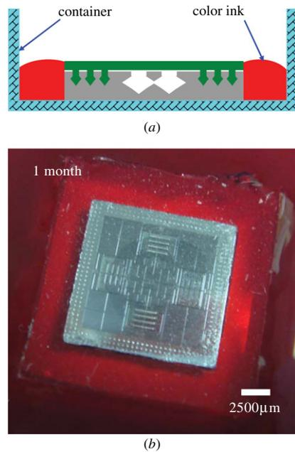
**Figure 13.** The preliminary liquid leakage test using color ink: (a) test setup and (b) no leakage occurred after testing for 1 month.
