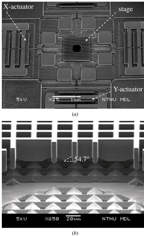
**Figure 7.** SEM micrographs of a typical fabricated device on the silicon substrate: (a) a 2D position stage and (b) the full release of the MEMS structure.
