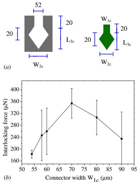
**Figure 11.** The measured interlocking force of connectors and sockets with press-fit designs.
