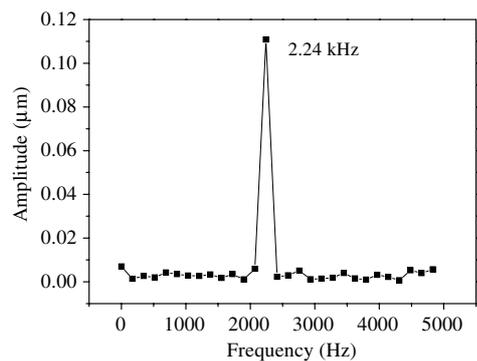
**Figure 12.** The measured frequency response of the 2D position stage after the package.
