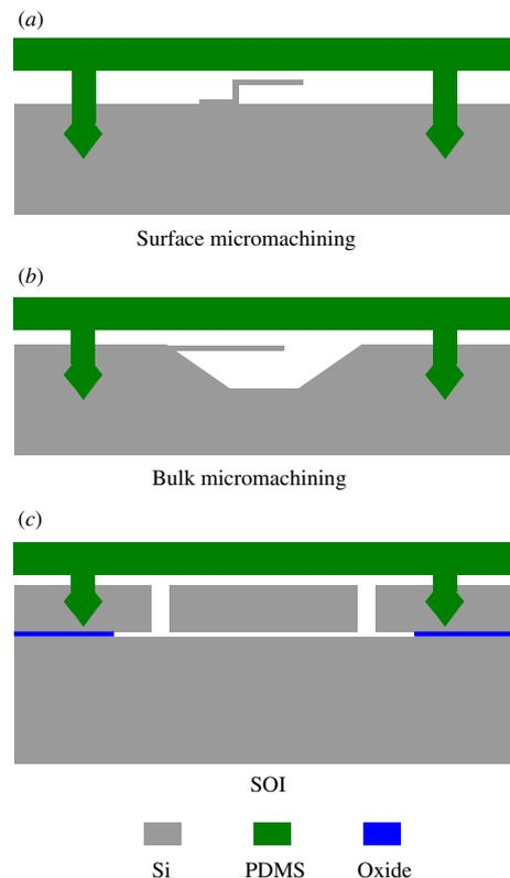
**Figure 2.** Various potential applications of the polymer cover for (a) surface, (b) bulk and (c) SOI micromachined devices.
