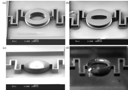
Fig. 4. Typical fabricated devices. Asymmetric type tunable lens with aperture radius of (a)  $X/Y = 200 \mu\text{m}/150 \mu\text{m}$ , (b)  $X/Y = 200 \mu\text{m}/75 \mu\text{m}$ . (c), (d) Side view and top view of lens after PDMS dispensing.
