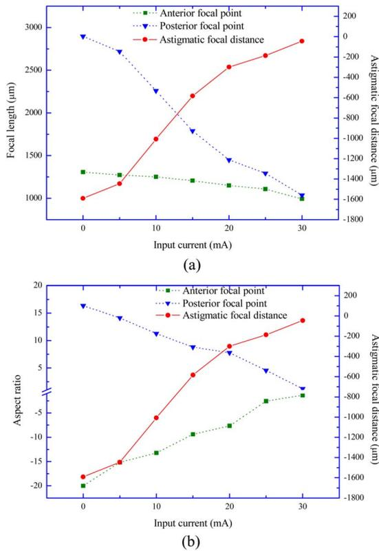
Fig. 5. Measurement results of astigmatism versus input current at wavelength = 632.8 nm. (a) Focal length of two focuses and AFD (negative sign indicates that the anterior focal spot is vertical-shaped), and (b) aspect ratio of focal spots changes with input current.
