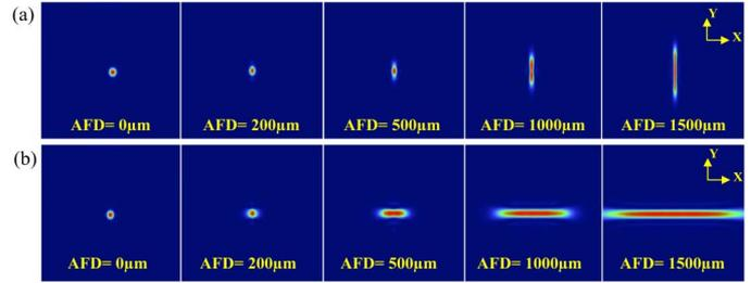
Fig. 3. Simulated (a) anterior and (b) posterior focal spots with increasing astigmatism for aperture radius of  $X/Y = 3/2$ . The AFD from left to right are 0, 200, 500, 1000, and 1500  $\mu\text{m}$ , respectively. (Wavelength = 632.8 nm).
