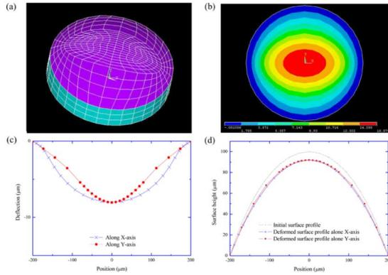
Fig. 2. Simulation of lens profile change under temperature change of 100 °C. (a) FEM model of PDMS lens and conducting ring; (b) contour plot of asymmetric surface deflection; (c) deflection along  $x$ - and  $y$ -direction; and (d) lens surface profiles before and after temperature change.
