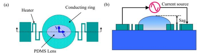
Fig. 1. Schematic of thermal tunable microlens. (a) Top view and (b) side view.
