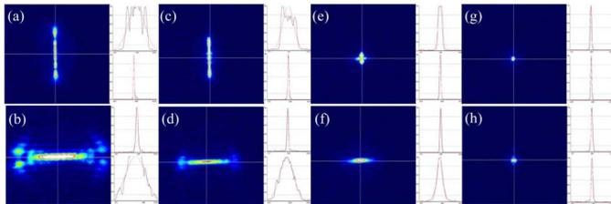
Fig. 6 Measured anterior and posterior focal spots at different driving current of (a), (b) 0 mA, (c), (d) 15 mA, (e), (f) 25 mA, and (f), (g) 30 mA.
