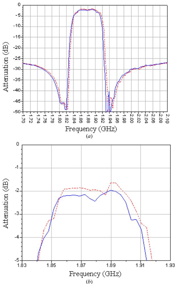
**Figure 11.** Temperature stability for a microcapped filter. The dashed line represents the filter measured at  $-30\text{ }^{\circ}\text{C}$  and the solid line represents the filter measured at  $85\text{ }^{\circ}\text{C}$ .
