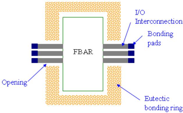
**Figure 3.** Schematic view of a eutectic bonding ring and interconnection lines.
