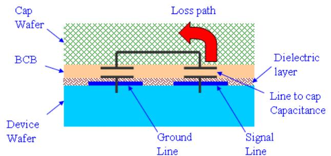
**Figure 5.** RF signal leakage from signal lines into ground through the microcap.
