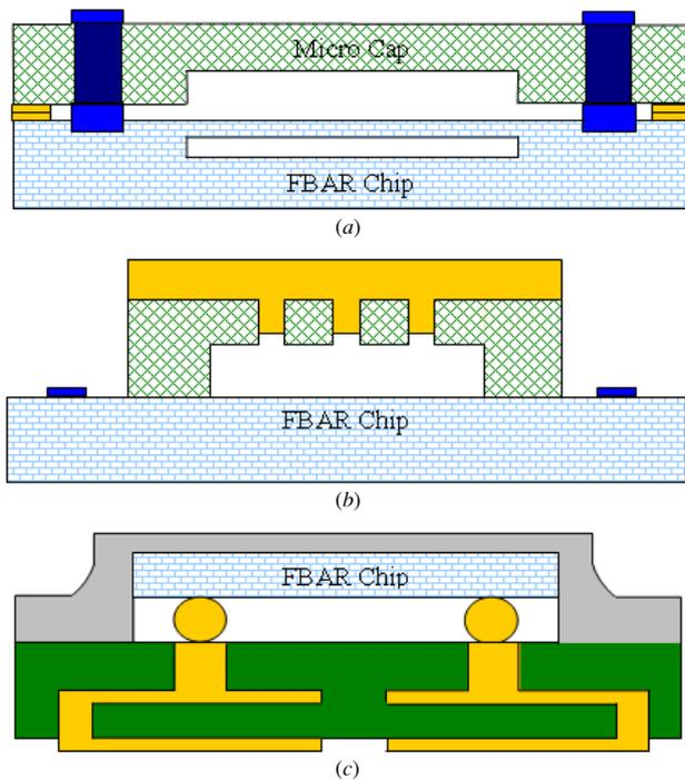
**Figure 1.** Schematic view of existing chip-scale packages for FBAR filters: (a) microcap with through-wafer interconnect, (b) photo-epoxy microcap, (c) flip chip on LTCC.
