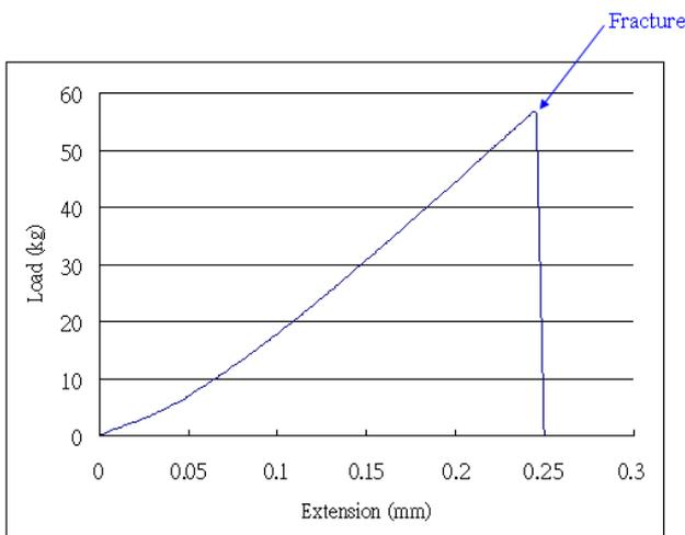
**Figure 9.** Tensile test result for BCB bonded wafers.
