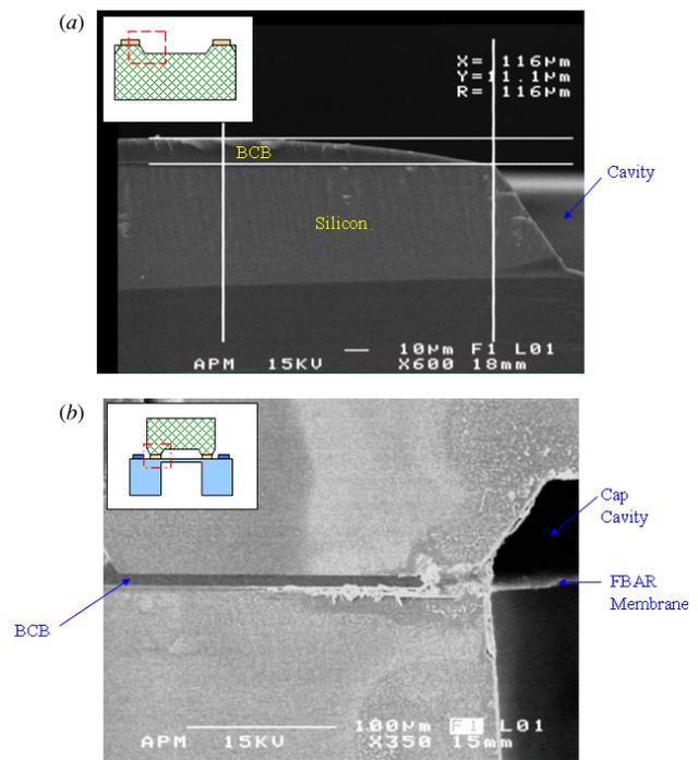
**Figure 4.** Cross-section SEM photo of a BCB bonding ring: (a) after photolithography, (b) after bonding.
