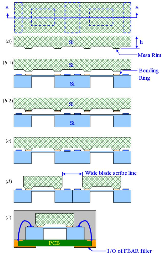
**Figure 2.** Process flow of the microcapped FBAR fabricated by the standard wafer saw method.
