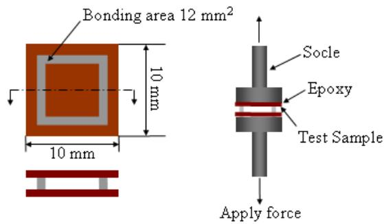
**Figure 8.** The experiment set-up for evaluation of bond strength. The sample was under a tensile test.
