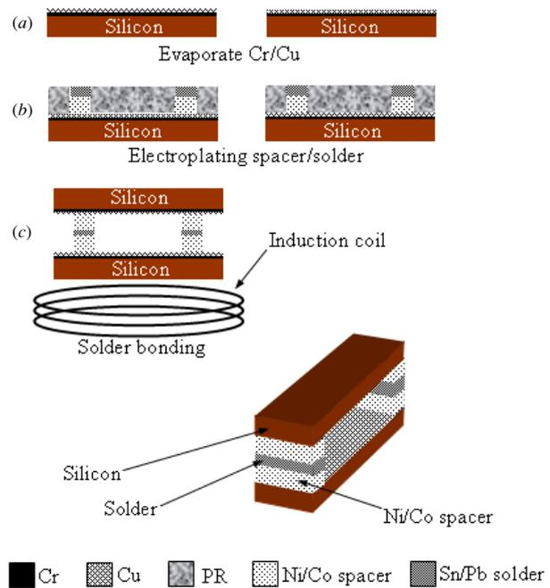
**Figure 2.** The concept and fabrication process for the present study.
