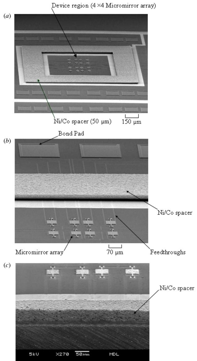
**Figure 5.** The SEM photographs of the integration of surface micromachined devices and the spacer (a) a  $4 \times 4$  mirror array inside the  $50 \mu\text{m}$  height Ni/Co spacer, (b) conducting wires and bonding pads of mirrors and (c) the microscopic section of the bonding region.
