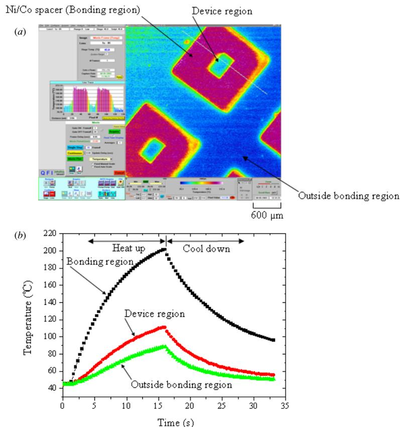
**Figure 7.** The measured temperature of the test sample during induction heating (a) spatial distribution, and (b) temporal distribution.
