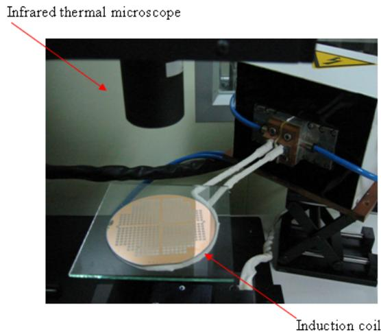
**Figure 6.** The experiment set-up in this study for induction heating. The sample was placed on top of a magnetic coil. The temperature distribution of the sample was inspected by an infrared microscope.
