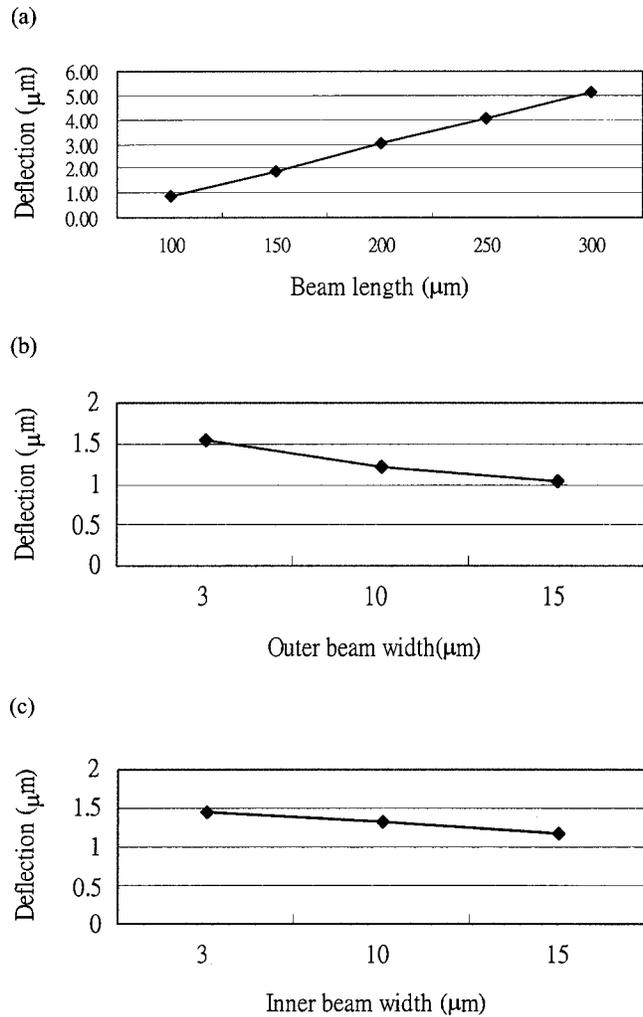
**Fig. 2** Geometric dimensions of the actuator: (a) deflection versus beam length, (b) deflection versus outer beam width, and (c) deflection versus inner beam width.
