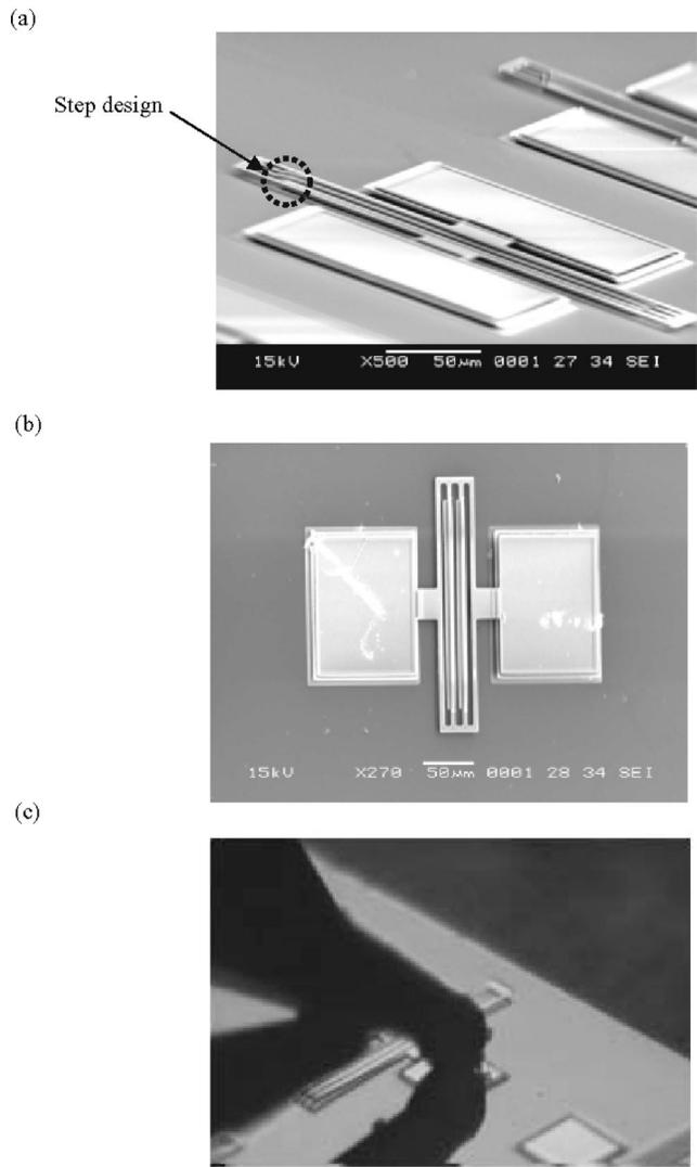
**Fig. 5** (a) The perspective view of the proposed thermal actuator, (b) the top view of the actuator, and (c) the actuated state of the actuator.
