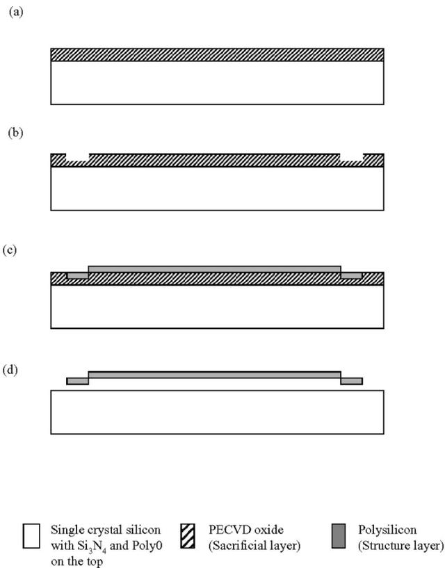
**Fig. 4** Fabrication processes of the proposed thermal actuator: (a) PECVD oxide deposition as the sacrificial layer, (b) pattern oxide to form dimple and anchor areas, (c) deposition LPCVD poly-Si as the structure layer, and (d) etching oxide to release the structure layer.
