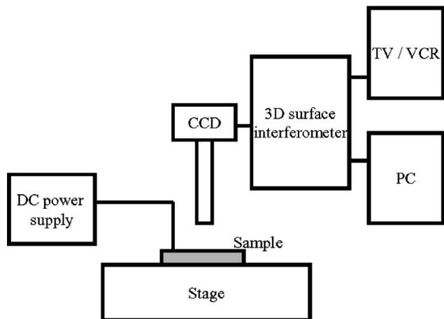
**Fig. 6** The experimental setup of the 3-D optical interferometer.
