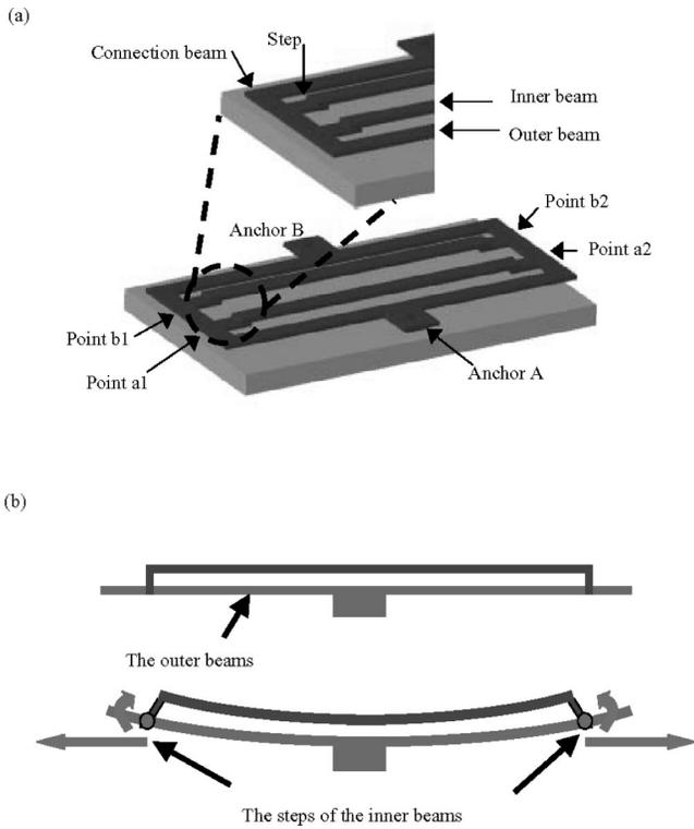
**Fig. 1** (a) The schematic drawing of the single-layer electrothermal actuator. (b) The illustration of the step design allows the outer beams to bend upward while the outer beams were heated.
