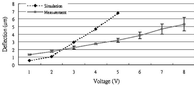
**Fig. 8** Variation of the deflection amplitude of the actuator with the driving voltage from 1 to 8 V dc.
