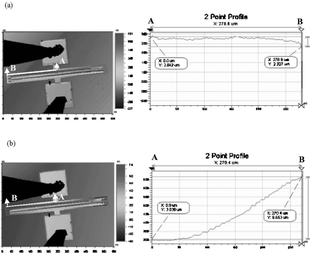
**Fig. 7** The static deflection of the actuator measured by the interferometer (a) when the driving voltage was 0 V dc and (b) when the driving voltage was 6 V dc.
