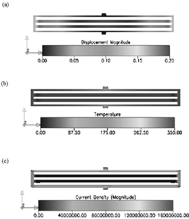
**Fig. 3** Simulation results of (a) upward deflection magnitude, (b) temperature, and (c) current density, for the driving voltage 3 V dc.
