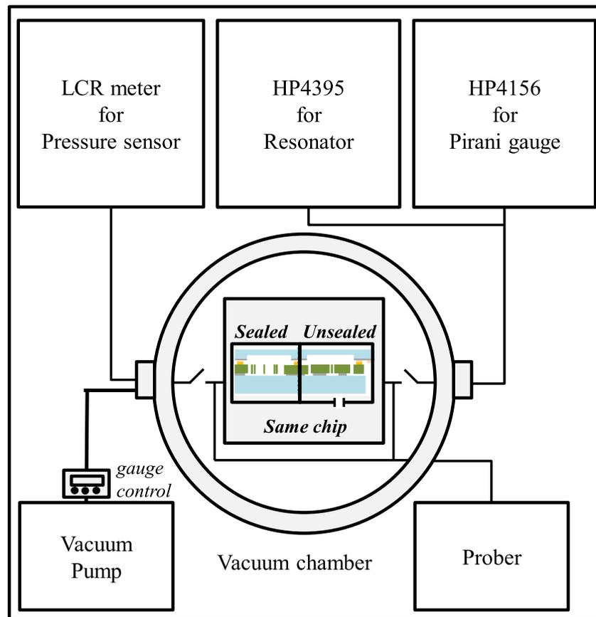
**Figure 9.** Schematic of the test setup including the PCC to accommodate the 8-inch wafer, manual probers, and three peripheral measurement tools for the signal extraction of different pressure sensitive devices such as, HP4156 for the resistance change (micromachined Pirani gauge), HP4395 for the impedance change (mechanical resonator), and LCR meter for the capacitance change (pressure sensor).
