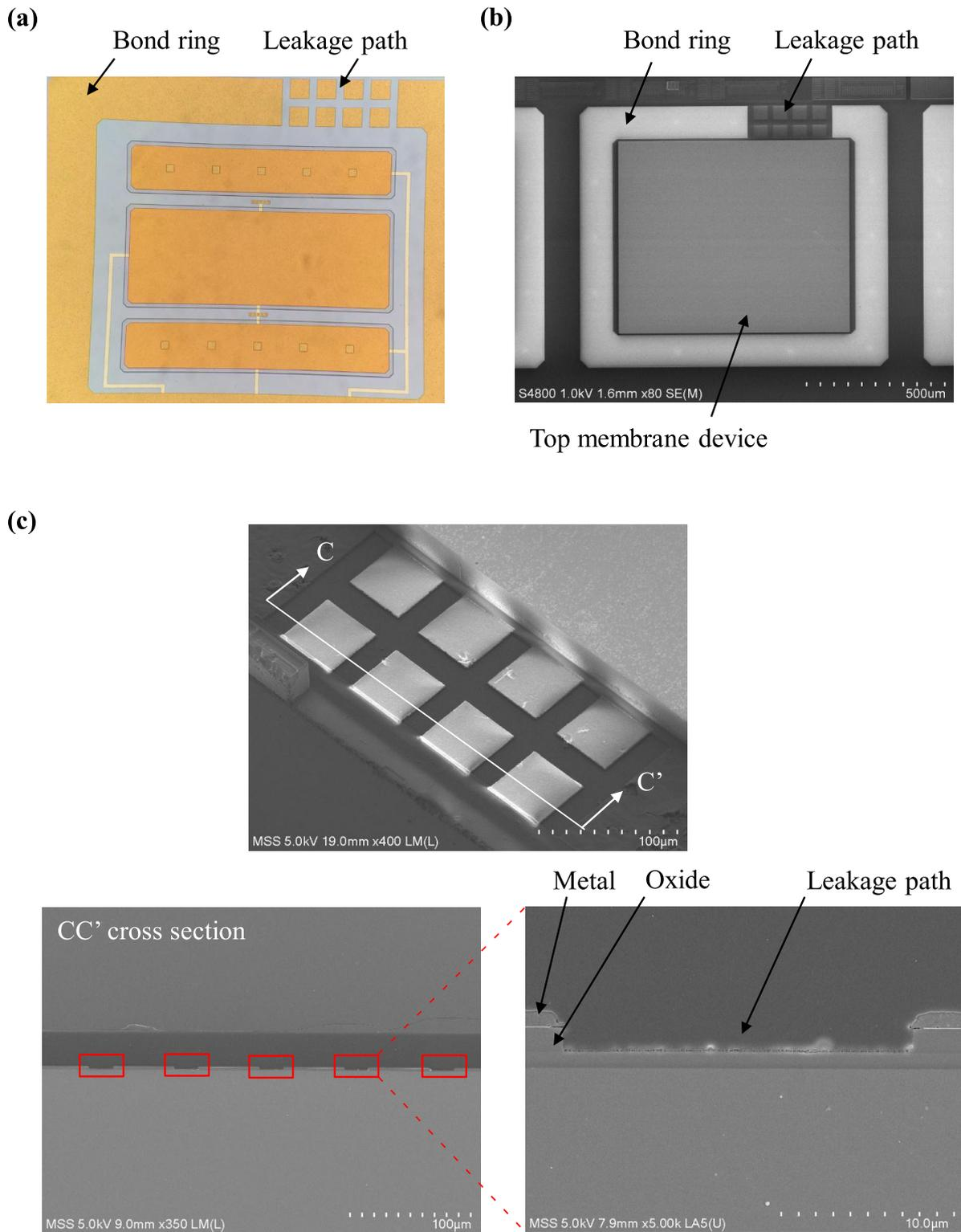
**Figure 7.** SEM micrographs of the inline process observation (a) the result after the process in figure 6(b) to show the exposed metal layer for bonding ring and the area without metal film is defined as the leakage path for the unsealed chamber, (b) the result after the process in figure 6(e) to show the bonding ring and the MEMS device before wafer eutectic bonding process, and (c) the zoom-in and cross-section views of the leakage path.
