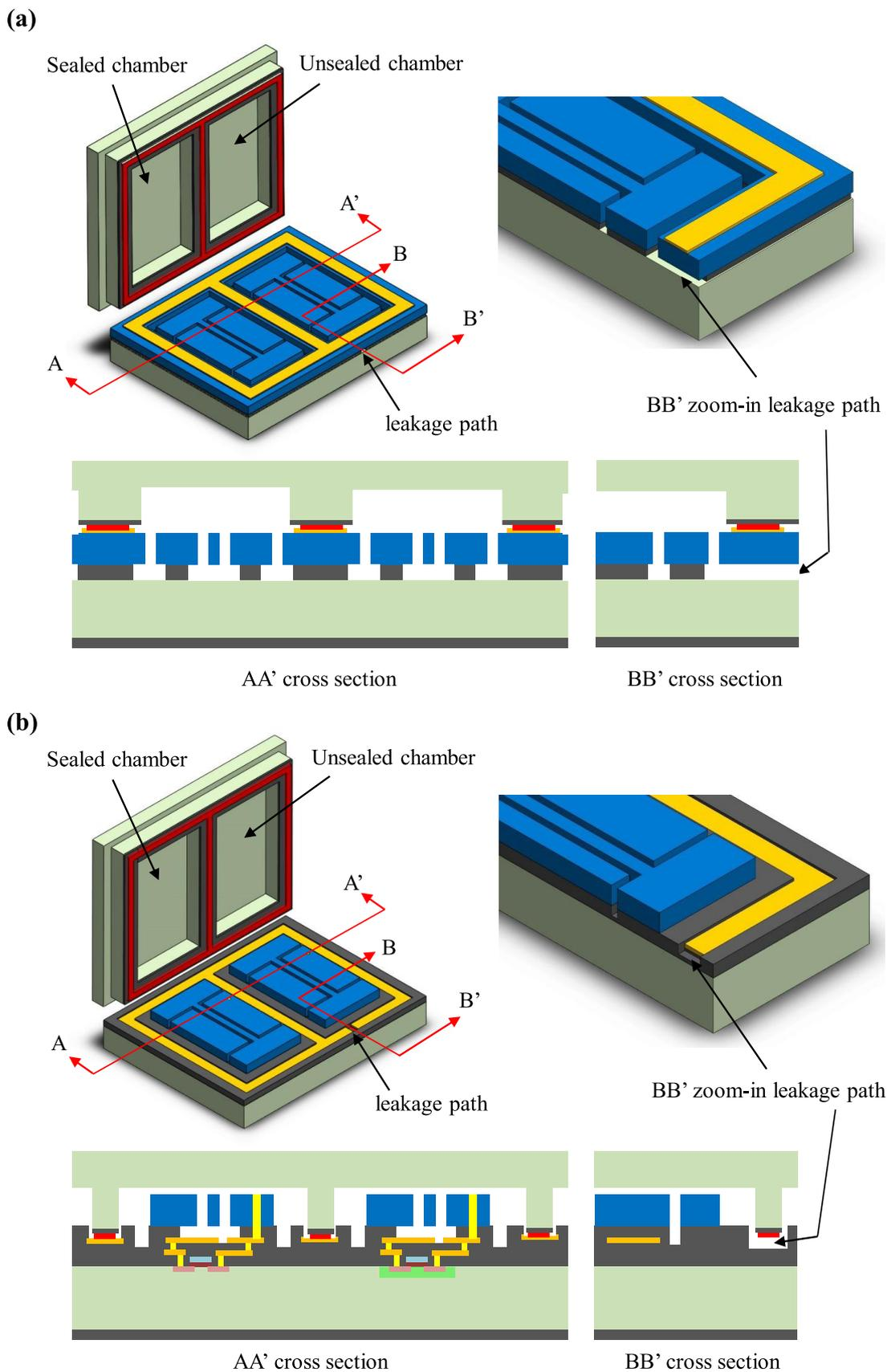
**Figure 2.** Extending the existing BOD and BOC platforms without additional process steps to realize sealed and unsealed chambers by using the proposed leakage path designs, (a) the leakage path on oxide layer is proposed for the BOD platform, and (b) the leakage path on the metal/oxide layers is proposed for the BOC platform.
