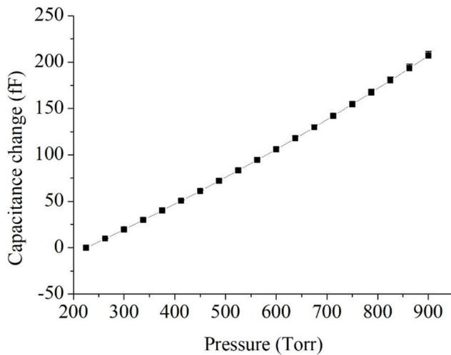
**Figure 12.** The functional tests of the capacitive pressure sensor encapsulated inside the unsealed chamber fabricated by the BOC platform. The sensing signals varying with vacuum conditions of PCC demonstrates that the present approach enables the BOC platform to integrate motion and environmental hubs.
