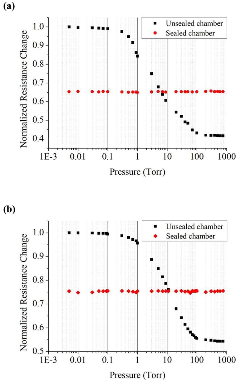
**Figure 10.** Typical measurement results of the micromachined Pirani gauge to show the normalized resistance change versus different pressure conditions of PCC for the unsealed and sealed chambers fabricated by (a) BOD platform, and (b) BOC platform.
