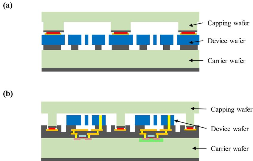
**Figure 1.** Silicon above CMOS foundry platforms, (a) the Bond on Device layer (BOD), and (b) the bond on carrier substrate scheme (BOC).
