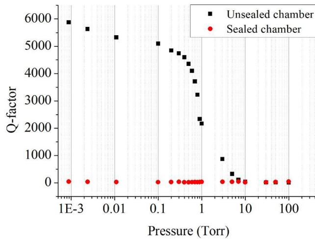
**Figure 11.** Typical measurement results of the mechanical resonator fabricated by the BOD platform, (a) the frequency response of resonator encapsulated inside a sealed chamber with a pressure of 10 Torr, and the quality factor determined from the measurement is 30, (b) quality factors respectively extracted from devices in unsealed and sealed chambers with different PCC pressure conditions.
