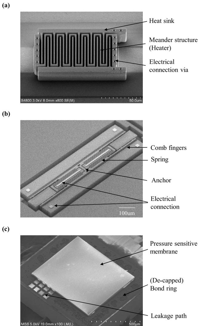
**Figure 8.** The three pressure sensitive sensors fabricated and embedded in the chambers to evaluate the approaches presented in this study, (a) micromachined Pirani gauge, (b) mechanical resonator, and (c) capacitive pressure sensor.
