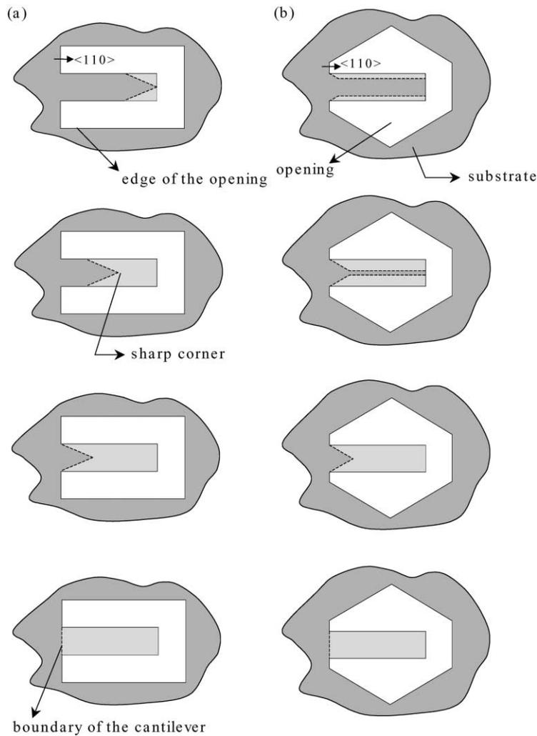
Fig. 5. Undercut process of a microcantilever on the (a) (1 1 1); and (b) (1 0 0) oriented wafer.
