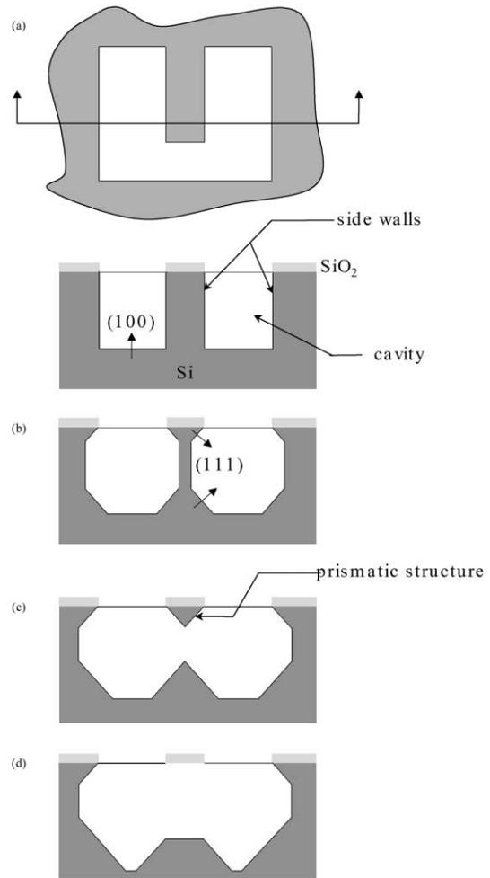
Fig. 9. Anisotropic etching prediction of cantilevers on (1 0 0) substrate when RIE depth is greater than  $w_0 \tan 54.7^\circ$ .
