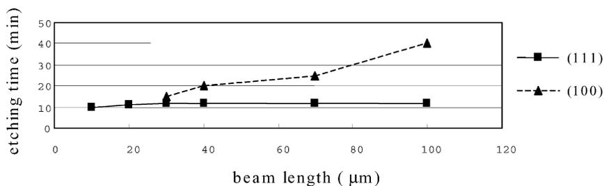
Fig. 6. The relation between beam length and etching time for cantilevers on both (1 0 0) and (1 1 1) substrates.
