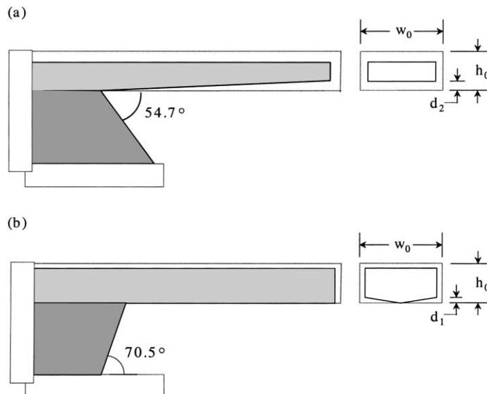
Fig. 7. Thickness variation of thin film on (a) (1 1 1); and (b) (1 0 0) oriented wafer after anisotropic etch of KOH.
