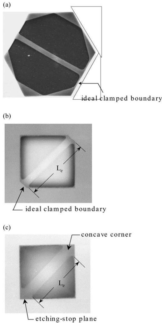
Fig. 3. Microbridges on the cavity of (a) (1 1 1) substrate with ideal clamped boundaries; (b) (1 0 0) substrate with ideal clamped boundary; (c) (1 0 0) substrate with concave corner.
