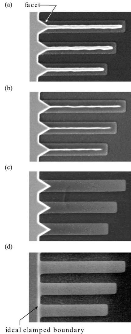
Fig. 4. OM photographs of microcantilever undercut process on (1 1 1) wafer when etch time is (a) 4; (b) 5; and (c) 12 min.
