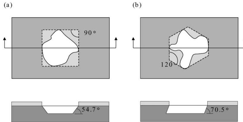
Fig. 1. Top view and side view of {111} planes in both (a) (100); and (b) (111) oriented silicon wafers.
