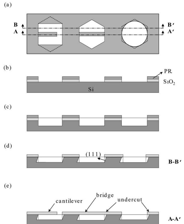
Fig. 2. Fabrication processes of structures on (111) oriented Si wafer.
