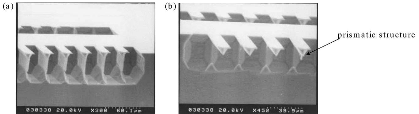
Fig. 10. SEM photos of undercut process for cantilevers on (1 0 0) substrate after Si RIE.
