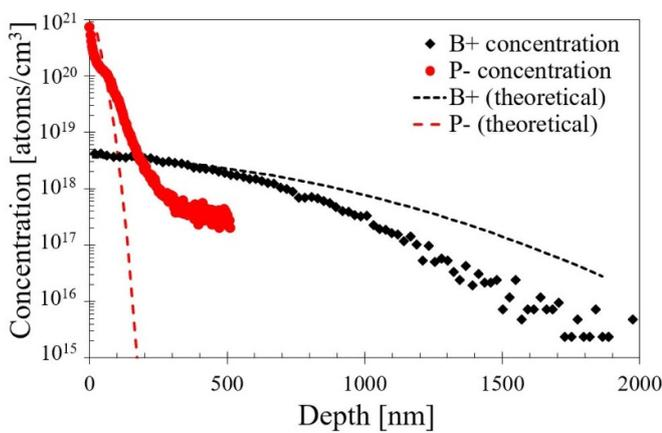
**Figure 6.** Dopant concentration profile on buried piezoresistor by SIMS analysis.
