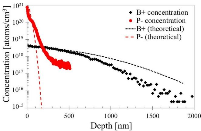
**Figure 6.** Dopant concentration profile on buried piezoresistor by SIMS analysis.
