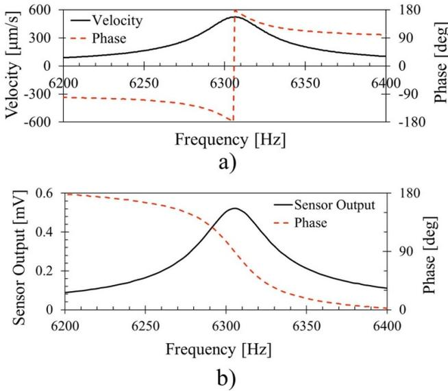
**Figure 8.** Dynamic evaluation of the device using (a) LDV and (b) fabricated buried piezoresistor.
