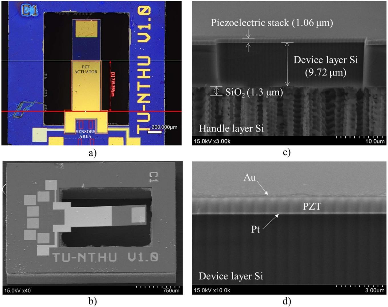
**Figure 5.** Finished cantilever test device. (a) Picture by optical microscope. (b) SEM picture. (c) Cross section on actuator area. (d) Close-up of piezoelectric stack cross section.
