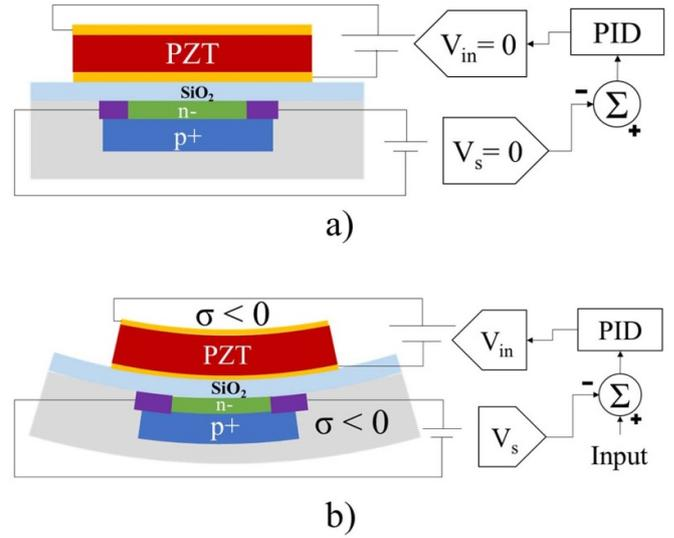
**Figure 1.** Design concept for PZT stable actuator. (a) Rest position, (b) actuation with feedback control system.
