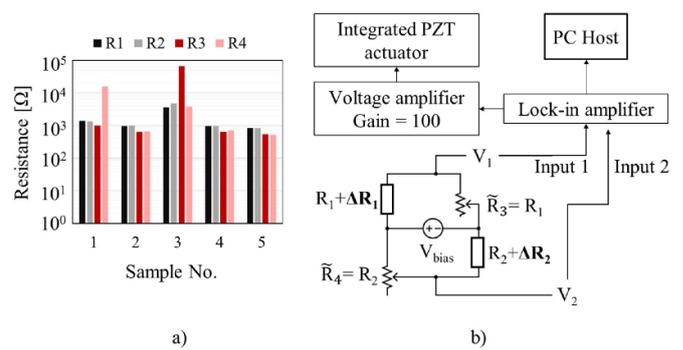
**Figure 7.** Buried piezoresistor evaluation. (a) Measured resistance of the four on-chip piezoresistors by multimeter for 5 different chips. (b) Experimental setup for sensor evaluation, showing the modified Wheatstone bridge to overcome the resistance mismatch between the on-chip piezoresistors.
