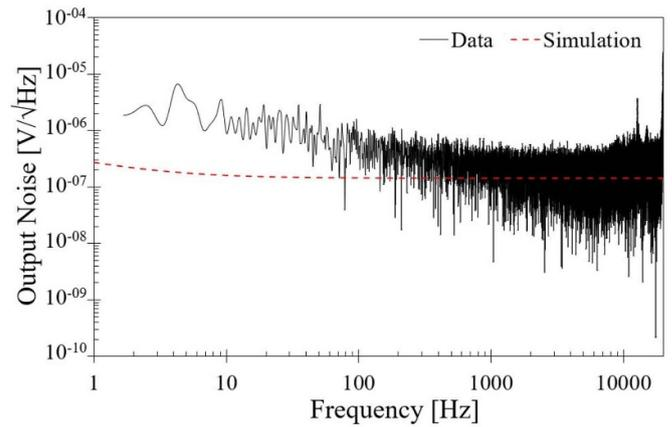
**Figure 10.** Electrical noise of output signal.
