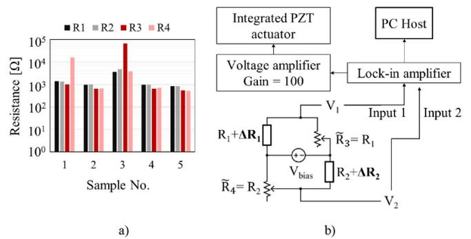
**Figure 7.** Buried piezoresistor evaluation. (a) Measured resistance of the four on-chip piezoresistors by multimeter for 5 different chips. (b) Experimental setup for sensor evaluation, showing the modified Wheatstone bridge to overcome the resistance mismatch between the on-chip piezoresistors.
