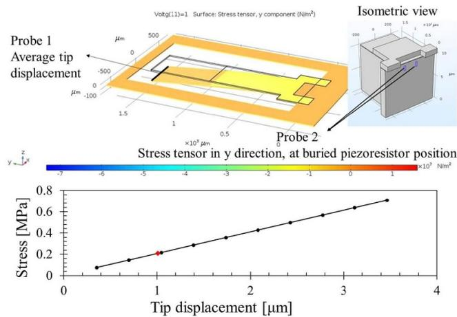
**Figure 3.** Static analysis by FEA. Model indicating probes position (top) and average stress in y direction at buried piezoresistor position (bottom).
