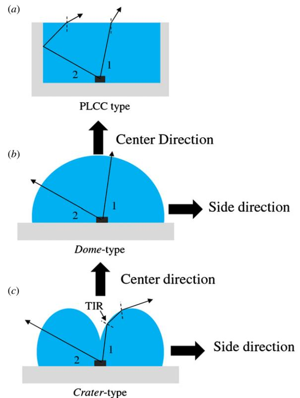
Figure 2. Light progressing in three types of package structures: (a) PLCC type, (b) dome-type, and (c) crater-type.
