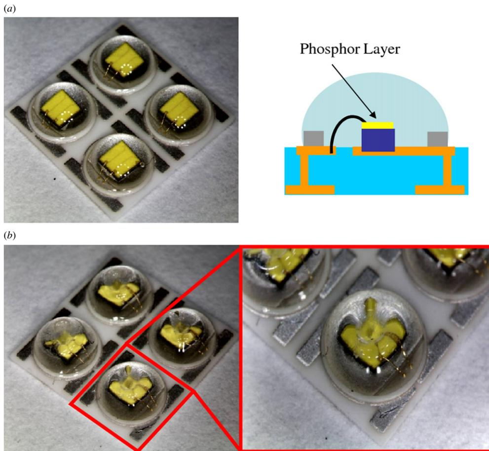
**Figure 9.** Typical fabrication results of white light LED, (a) dome-type package, and (b) crater-type package.
