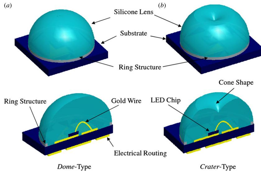
Figure 1. Design concept of the LED package and their cross sectional views: (a) dome-type design and (b) crater-type design.
