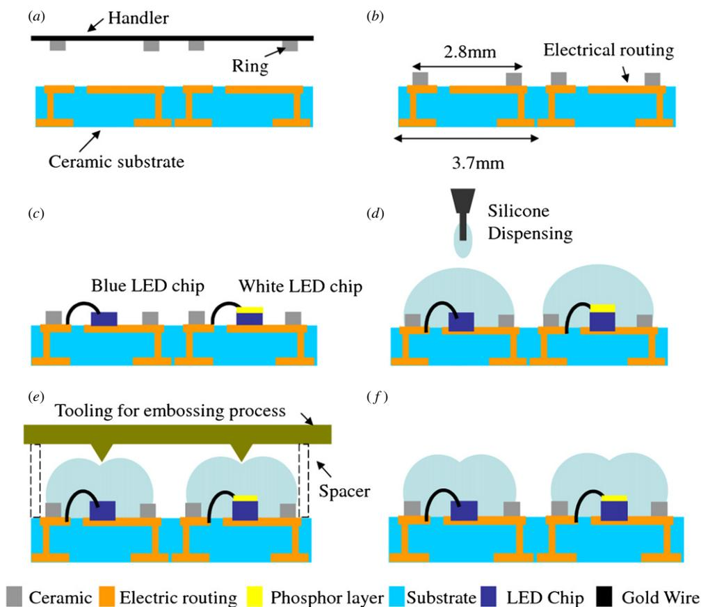
**Figure 5.** Fabrication and packaging steps, (a) ring type micro structure bonding on ceramic substrate, (b) ceramic substrate with ring type micro structure and electrical routing, (c) LED chip bonding and wire bonding, (d) silicone dispensing to achieve the dome-type package, and (e), (f) an additional embossing process to implement the crater-type package.
