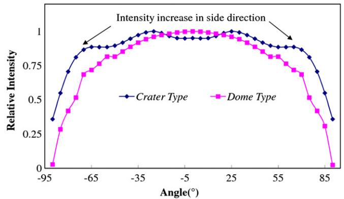
**Figure 4.** The intensity distribution of spatial radiation in the inner surface of hemisphere shell.
