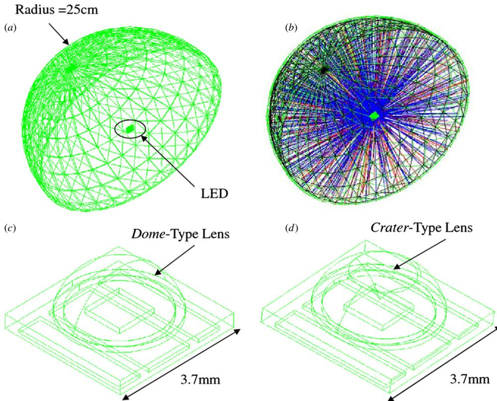
**Figure 3.** Model for optical simulation, (a) the package is arranged in the center of hemisphere shell, (b) light emit to the inner surface of hemisphere shell, and (c) dome-type package, and (d) crater-type package.
