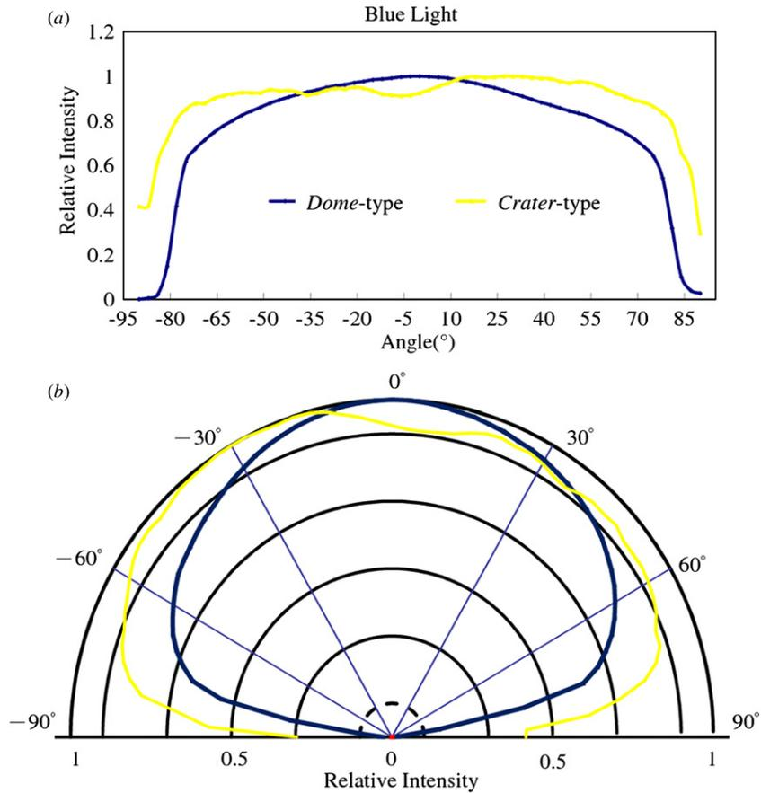
**Figure 12.** Measurement results of spatial radiation patterns for packaged monochromatic blue light LED, (a) rectangular coordinates and (b) polar coordinates.
