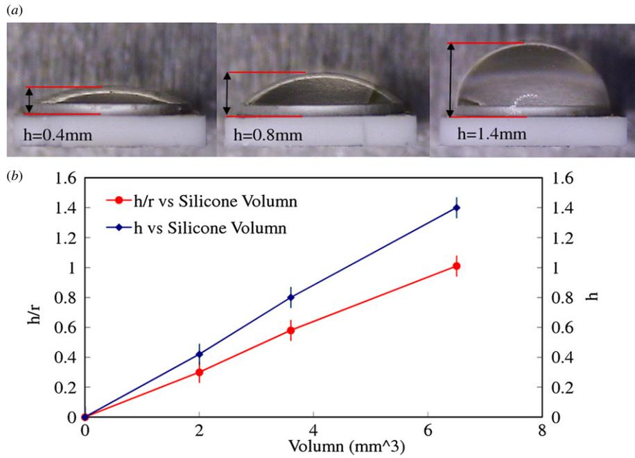
**Figure 7.** Dome-type lens shape modulated by the volume of dispensed silicone, (a) various lens heights, (b)  $h$  and  $h/r$  versus silicone volume by measurements.
