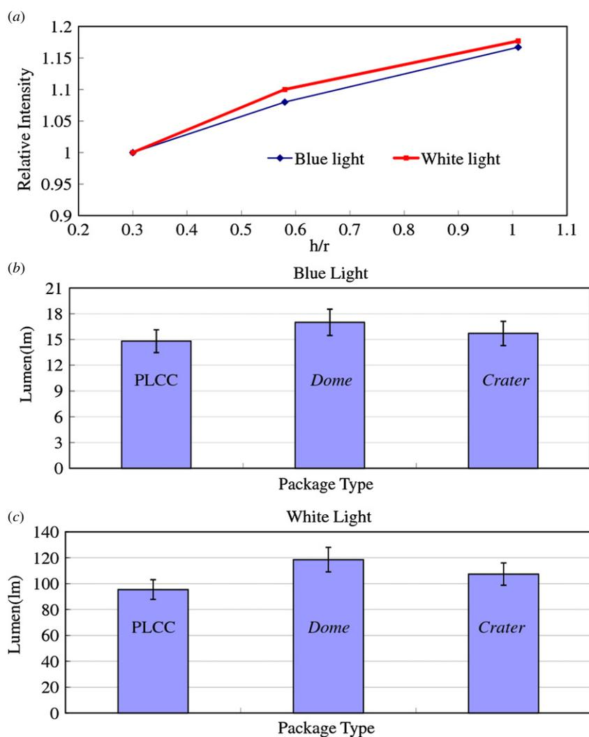
**Figure 11.** Measurements of LED package, (a) relative intensity versus  $h/r$  for dome-type package, and (b), (c) luminous flux of monochromatic blue light and white light LED chips packaged in three different approaches.
