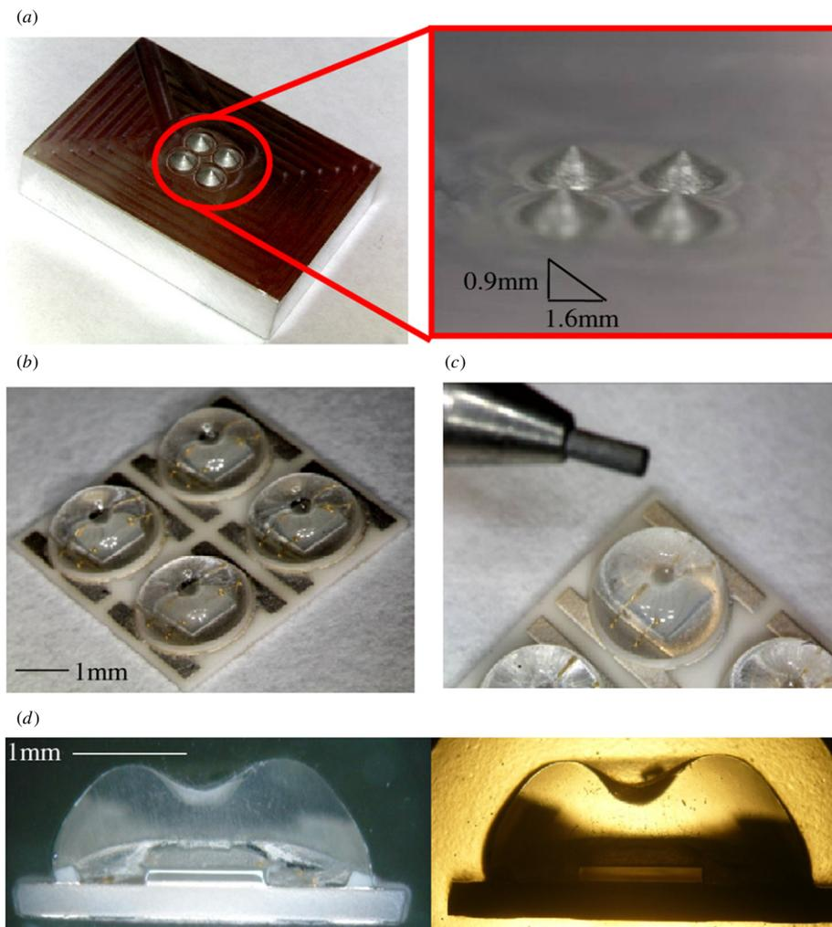
**Figure 8.** Typical fabrication results of crater-type package, (a) tooling used for embossing process, (b) and (c) crater-type package, (d) cross-sections of crater-type lens.
