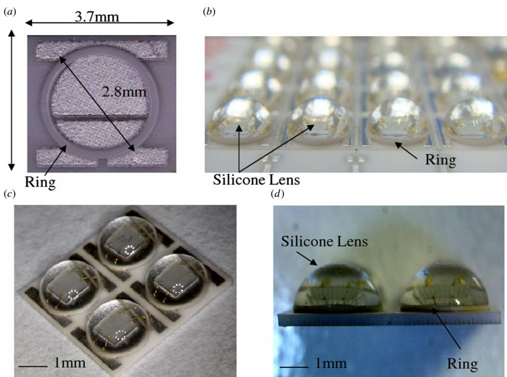
**Figure 6.** Typical fabrication results of (a) ceramic substrate, (b) dome-type package, and (c), (d) the zoom-in top and side views of dome-type package.
