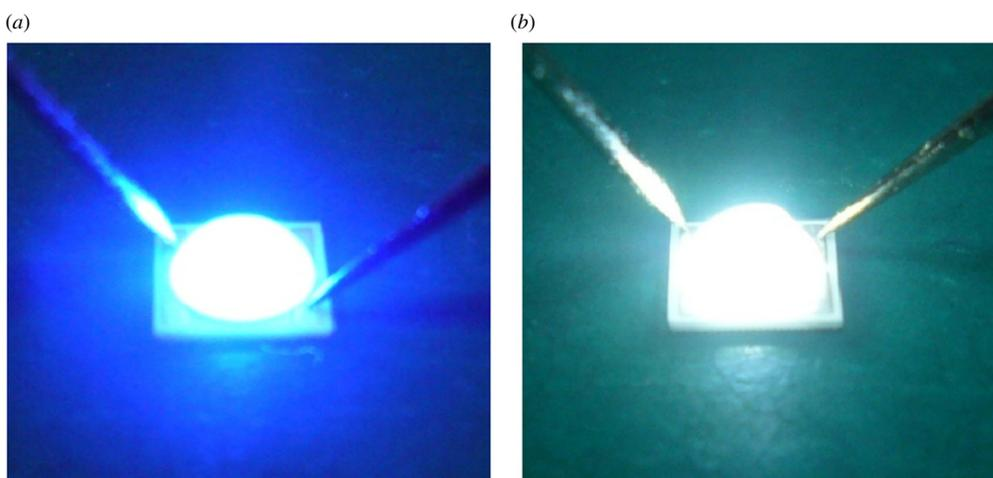
**Figure 10.** Light emitting from dome-type package with (a) monochromatic blue light LED chip, and (b) white light LED chip.
