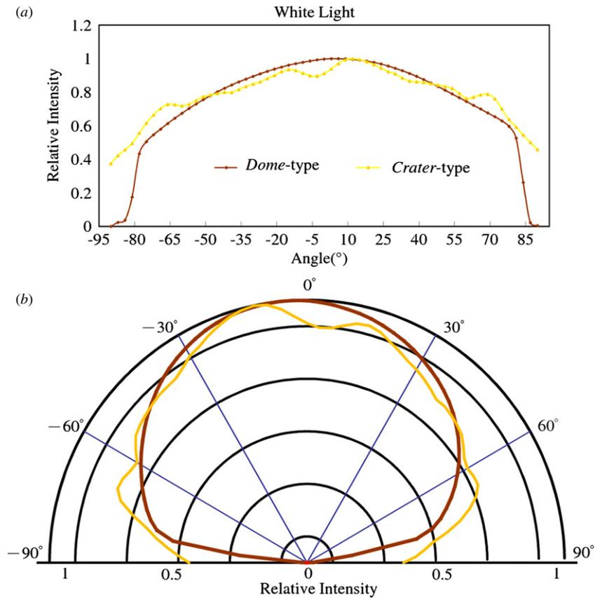
**Figure 13.** Measurement results of spatial radiation patterns for packaged white light LED, (a) rectangular coordinates and (b) polar coordinates.
