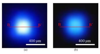
Fig. 10. Captured light intensity patterns of micro-LED arrays. (a) With sapphire microreflector. (b) With common-N interconnection.
