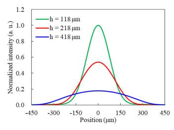
Fig. 16. Analyzed light intensity distribution for different sapphire substrate thicknesses.
