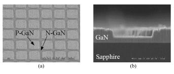
Fig. 8. (a) Accomplished micro-LED array with common-N interconnection. (b) Exposure N-GaN part after GaN etching.
