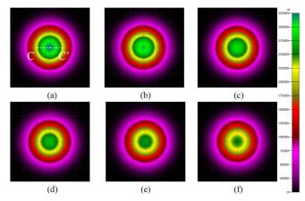
Fig. 12. Simulated light intensity pattern for sapphire microreflectors with different inclination angles. (a)  $65^{\circ}$ . (b)  $70^{\circ}$ . (c)  $75^{\circ}$ . (d)  $80^{\circ}$ . (e)  $85^{\circ}$ . (f)  $90^{\circ}$ .
