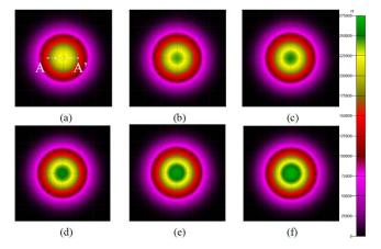
Fig. 3. Simulated light intensity pattern for micro-LED arrays with different sapphire microreflector thicknesses. (a) Common-N (reference array). (b) 5  $\mu$ m. (c) 10  $\mu$ m. (d) 15  $\mu$ m. (e) 20  $\mu$ m. (f) 25  $\mu$ m.
