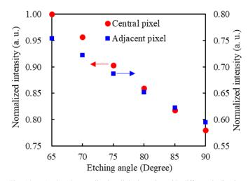
Fig. 14. Analyzed normalization light intensity with different inclination angles on sapphire microreflectors.
