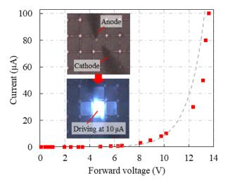
Fig. 9. Current–voltage (I - V) characteristic of the micro-LED pixel with sapphire microreflector and the operating condition.
