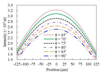
Fig. 13. Analyzed light intensity distributions with different inclination angles along C-C' line.
