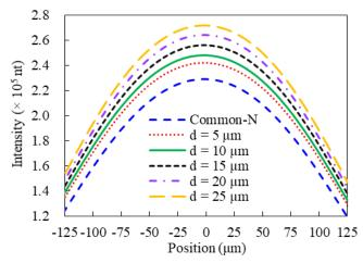
Fig. 4. Simulated light intensity distribution with different sapphire micro-reflector thicknesses along A-A' line.
