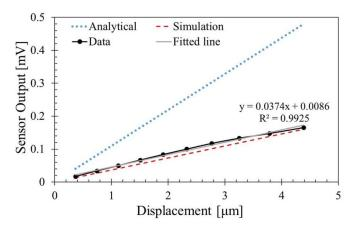
**Figure 9.** Sensitivity evaluation. Non-resonant actuation (9 kHz) at increasing unipolar voltage from 1 V to 10 V.
