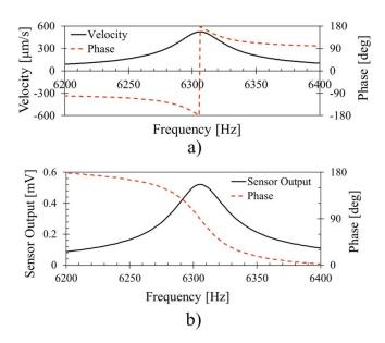
**Figure 8.** Dynamic evaluation of the device using (a) LDV and (b) fabricated buried piezoresistor.
