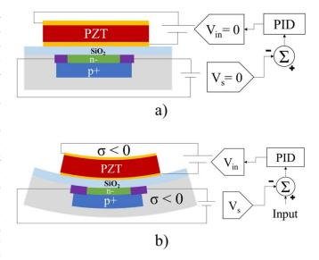
**Figure 1.** Design concept for PZT stable actuator. (a) Rest position, (b) actuation with feedback control system.
