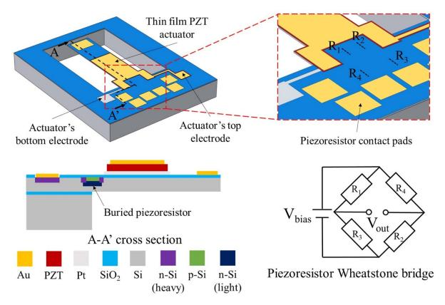
Figure 2. Device schematic. A 3D figure and cross section view of the device are shown on the left side. A close-up of the sensors area and electrical connection diagram are shown on the right side.
