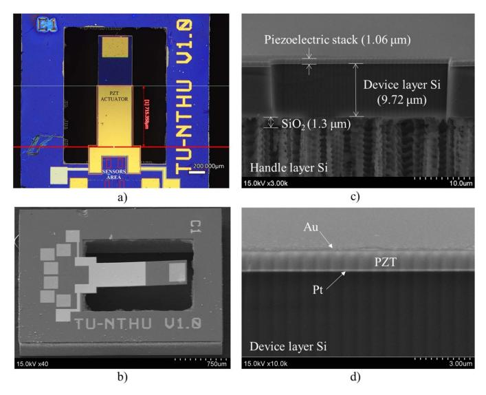
Figure 5. Finished cantilever test device. (a) Picture by optical microscope. (b) SEM picture. (c) Cross section on actuator area. (d) Close-up of piezoelectric stack cross section.
