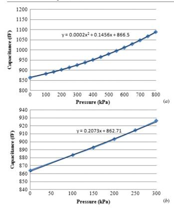
**Figure 7.** Capacitance versus pressure: (*a*) pressure range 0–800 kPa, (*b*) pressure range 0–300 kPa.
