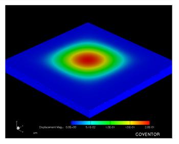
Figure 5. Simulated displacement distribution for an applied pressure of 300 kPa.
