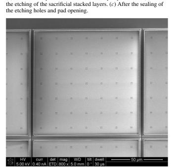
Figure 3. SEM (scanning electron microscope) photograph of the top view of the released membrane.
