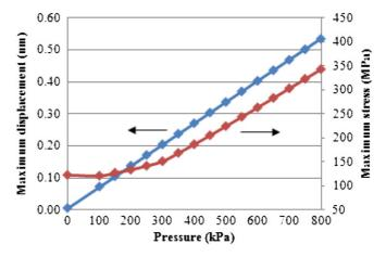
Figure 6. Relationship between displacement (left) and maximum stress (right).
