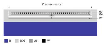
Figure 1. Cross-sectional view of the CMOS MEMS pressure sensor
