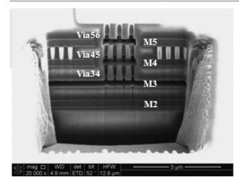
Figure 4. SEM photograph of the cross-sectional view of the released membrane.
