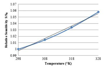
Figure 8. Pressure sensitivity versus temperature.
