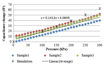
Figure 10. Measured results of the pressure sensor: dependence of capacitance change on applied pressure.
