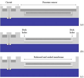
Figure 2. CMOS MEMS pressure sensor fabrication process flow: (a) after the completion of the CMOS and pad protection. (b) After
