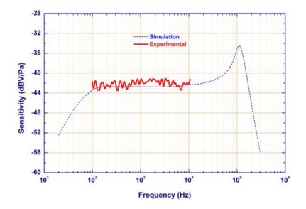
**Table 2.** Measured specifications of the packaged microphone.
